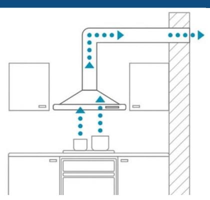
Kitchen & Bath Fans Must Exhaust Outside and Meet Airflow & Sound Limits
